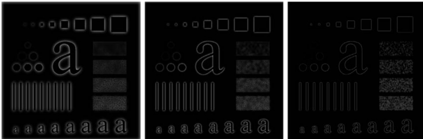
FIGURE 4.56 Results of highpass filtering the image in Fig. 4.41(a) using a GHPF with D_0 = 30, 60, and 160, corresponding to the circles in Fig. 4.41(b). Compare with Figs. 4.54 and 4.55.
